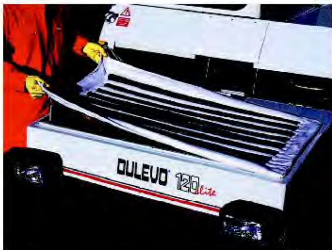
The filter system
