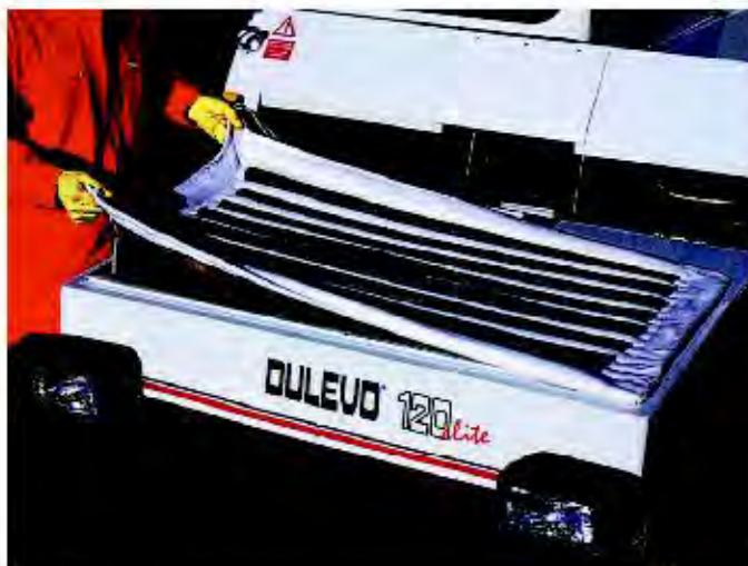
The filter system
