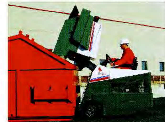
Emptying the waste hopper
