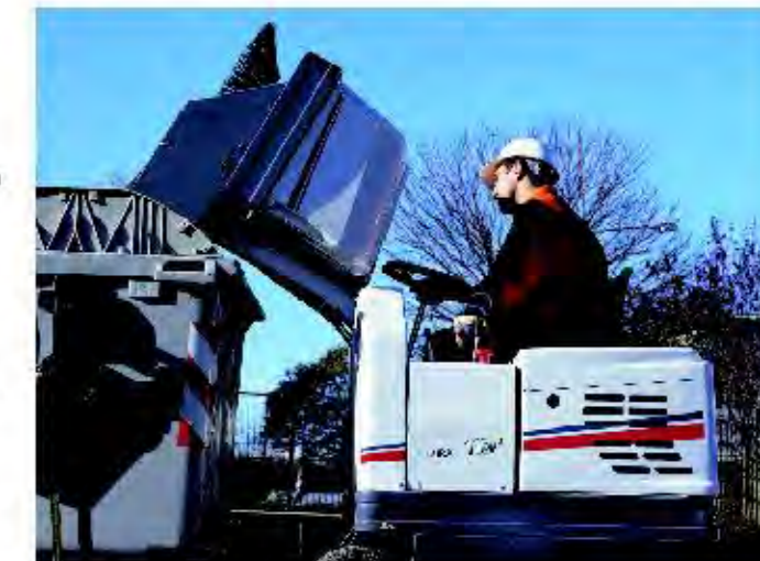
Emptying the waste hopper
